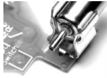
Push the motor up against mounting tabs
